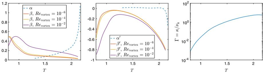
**Fig. 1** Dimensionless friction parameters  $\alpha$  and  $\beta$  (left),  $\alpha'$  and  $\beta'$  (centre) and  $\Gamma$  (right) as a function of temperature  $T$  and, for  $\beta$  and  $\beta'$ , typical vortex Reynolds numbers, defined as  $Re_{\text{vortex}} = |\mathbf{v}_{n\perp} - \dot{\mathbf{s}}|a_0/4v_n$
