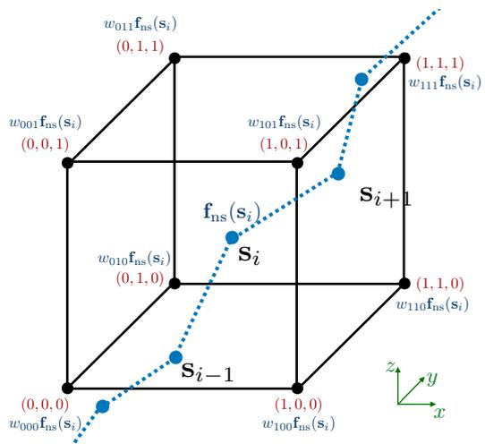
points of  $\mathbf{s}_i(t)$ . The force  $\mathbf{f}_{\text{ns}}(\mathbf{s}_i(t))$  exerted by the vortex line on the normal fluid has to be distributed among neighbouring points using weights  $w_{\zeta,\mu,\chi}$ , as shown schematically in Fig. 4.
