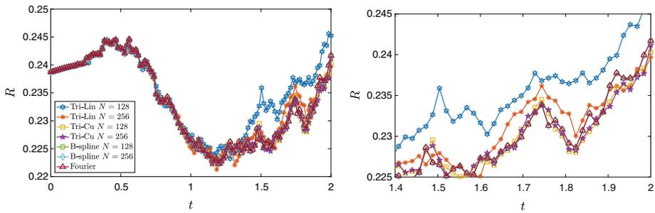
**Fig. 2** Temporal evolution of the average radius of a vortex ring for different interpolation schemes and normal fluid grid resolutions (arbitrary units). The right figure displays an enlargement of the left figure at late times to better judge the interpolation schemes
