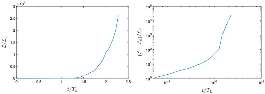
**Fig. 9** Left panel: Temporal evolution of the total vortex length  $\mathcal{L}$  resulting from a (initially perfect) vortex ring of length  $\mathcal{L}_0 = 2\pi R \approx 1.5$  in a turbulent normal fluid background. Right panel: relative increase of the vortex length during the initial stage
