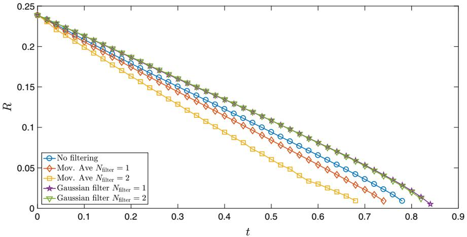
**Fig. 5** Temporal evolution of the radius of a vortex ring with in an initially uniform, quiescent normal fluid. The force acting on the normal fluid is distributed to the nearest neighbour point of the mesh. Different filtering procedures are tested
